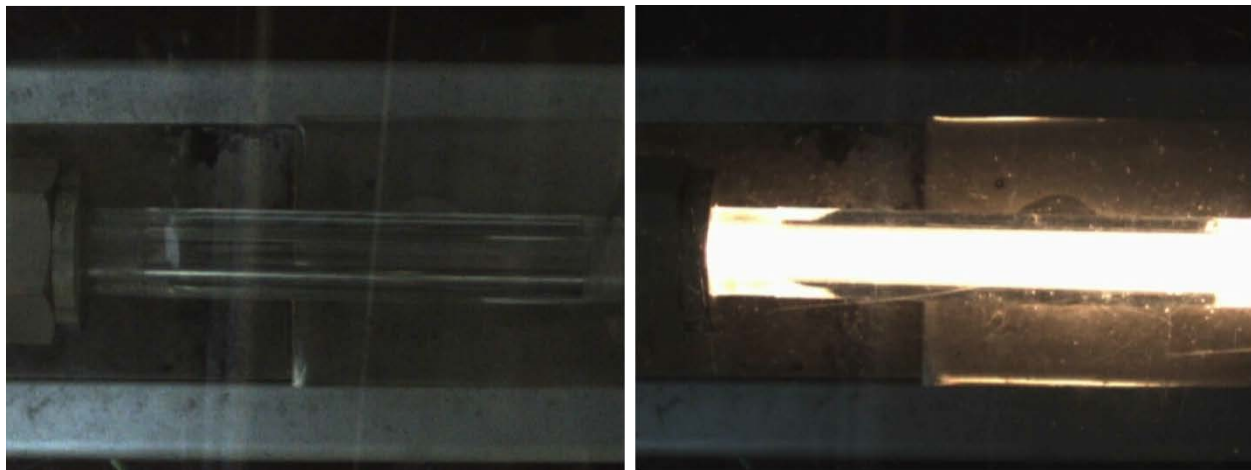
Figure 9: PMMA tube in feeding line before ignition (left) and after/during flashback (right)
