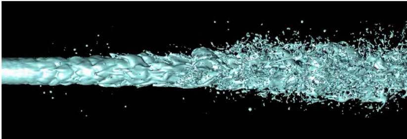
Figure 2.2.: Liquid jet surface and break-up results of DNS simulation [23]
